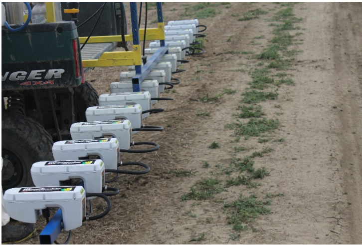
Figure 1: WeedSeeker sprayer with 16 LASC units for precision weed control in chemical fallow (2016).
