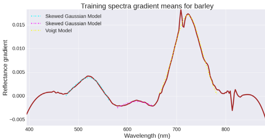
Figure 2. Gradient of the barley spectrum with a skewed Gaussian fit for 475-565 nm, a skewed Gaussian fit for 580-655 nm and a Voigt profile fit for 665-785 nm.
